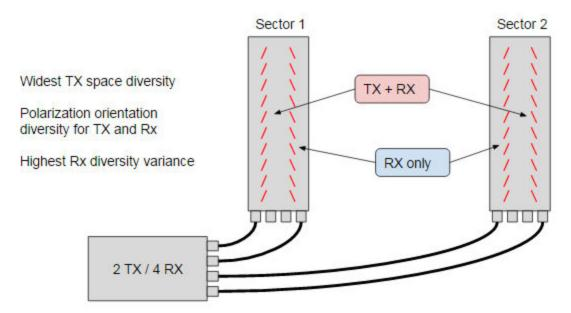
The future is about large-scale MIMO. MIMO is the amazing technology that allows multiple transmitters to send different streams of data at the same time on the same frequency generating a cacophony of interfering signals that a receiver can tease apart by knowing the channel function between each transmitter and receiver. There are consumer WiFi devices that do this with two streams.
