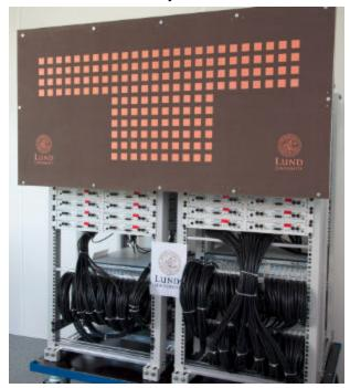
The TX and RX side each need to have at least as many antennas as streams. When talking to handheld mobile devices, which are too small for many antennas, MIMO is still beneficial because a base station can use its antenna to do beamforming to form the equivalent of a highly directional antenna aimed right at the mobile device.
