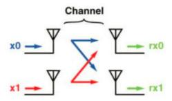
Kapela went over examples of very massive MIMO, greater than 100 streams. This seems like it would take an ideal channel with no correlation between the channel functions from each TX antenna to each RX antenna. Kapela explained that this is not necessary. The receiver can send feedback to the transmitter on the channel, so that the transmitter can precondition its transmissions favorably for MIMO.
